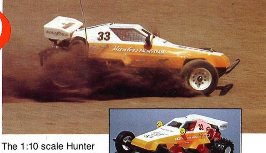
The 1:10 scale Hunter has independent double-wishbone front suspension, with swing arms
